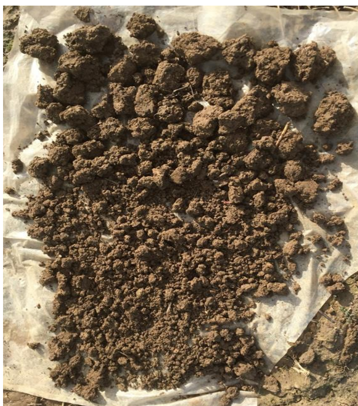
Figure 3. Assessment of soil structure and consistence (for VSA score) carried out pre-blackcurrants.
